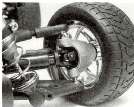
Plastic drive shafts power the Pirate 10 SR. The included tires don't come with foam liners and are a little squishy. I had to use off-road tire foam liners to firm them up.
