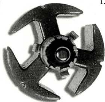
As you can easily see in this photo, the new Dirtinator 2's armature (above) is 25 percent thicker than the original's (right).
