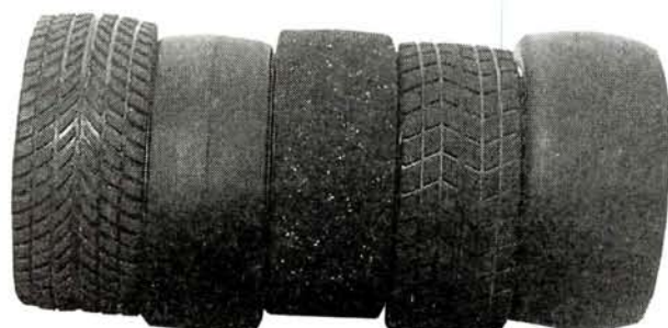
Different brands or types of tires may have different diameters. A one-way will eliminate any handling problems caused by tire size.
