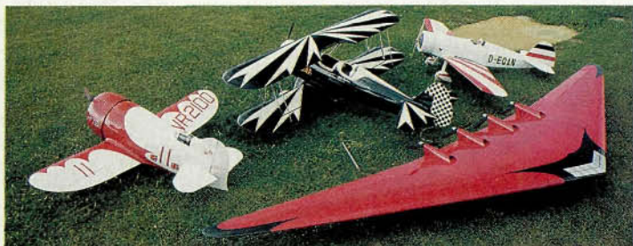
Keith Shaw brought these electric scale beauties to the September 1990 KRC Electric Fly (held annually in Quakertown, PA). From left to right, clockwise: Gee-Bee, 450 Stearman, Messerschmitt M-354 and "King Crimson" flying wing (powered by four Leisure ferrite 05 can motors and 28 Sanyo 1200mAh SCR cells).
