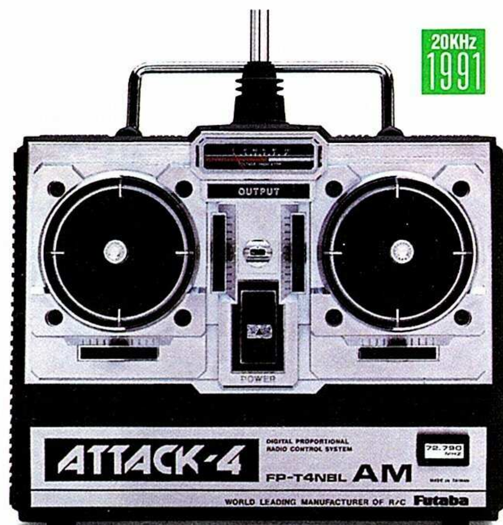
4NBL Attack S/4 Channel AM Aircraft system. R114H receiver, three S148 servos, servo reverse. Transmitter NiCd. 72 and 75 (surface) MHz.
