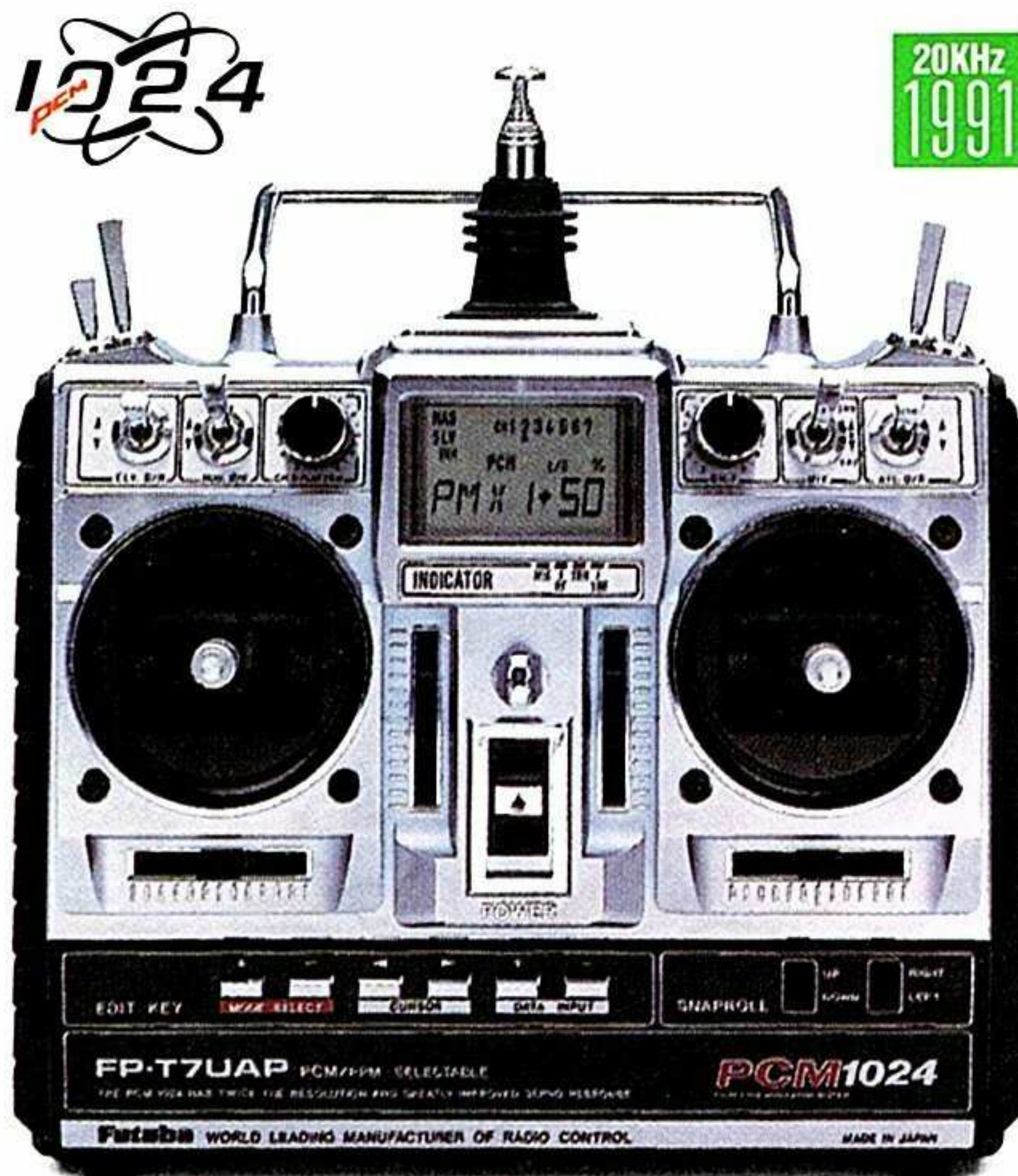
7UAP/7 Channel PCM 1024 Aircraft system. R129DP receiver, four S148 servos, computer LCD screen, ATV, dual rate, exponential, programmable mixing, timer, snap roll(4), servo reverse, memory, plug-in RF module, trainer system. All NiCd. 50 and 72MHz.
