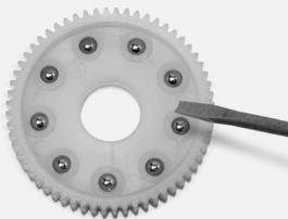
Insert the nine 1/8" balls into the main differential gear. Use a small screwdriver or knife to apply small amounts of lubricant both sides of the balls. Use a quality ball diff lubricant from your local hobby dealer. **DO NOT substitute ball diff lubricant with any other kind of grease or oil.** Also lubricate the inside of the diff gear with differential lubricant.
