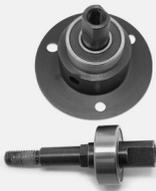
Test to be sure that your ball bearings or bushings fit smoothly over the diff shaft and housing shaft. It may be necessary to polish the shafts with 220-440 fine grit sandpaper, until the bearings or bushings slide on smoothly.
